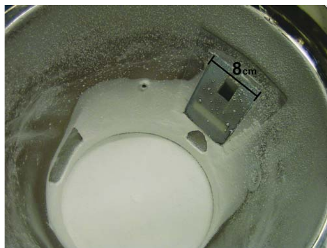
Fig. 5. On-line sampler in the granulation chamber
